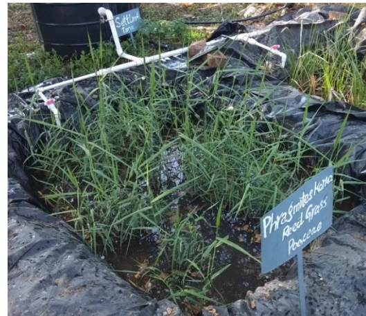
Fig. 3: Treatment of wastewater in Wetland with Phragmites karka
